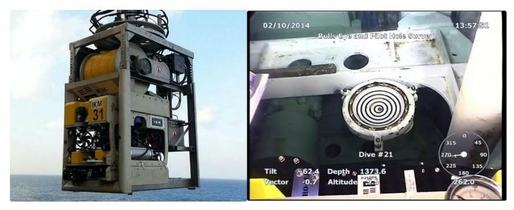
Our Mohican Inspection Class ROV system incorporates an enhanced propulsion system allowing it to continue working in high current conditions when other systems have to return to surface, providing a customer benefit of reduced vessel time and costs. The subCAN control system provides advanced diagnostics, precise vehicle control and reduced reactive maintenance.
