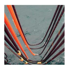
We can customize a maintenance program for the bulk-loading hoses with regular periodic inspections to determine whether the hose is suitable for continuing in service. Generally during maintence, a visual inspection of the hose and couplings is done for loose covers, kinks, bulges or soft spots which might indicate broken or displaced reinforcement; evidences of coupling failure. The hose may then be subjected to a hydrostatic test pressure if this is available.
