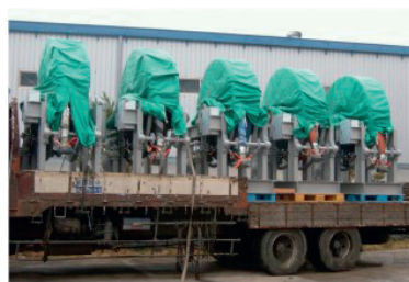
4" Couplings on hose reels for loading supply vessels with Methanol, diesel, drilling mud.
