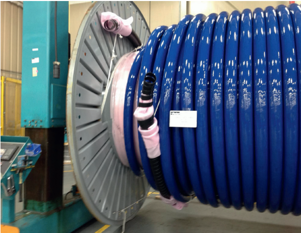
700 m BOP Control Umbilical with 101 lines delivered to a drilling rig in the UK sector.
