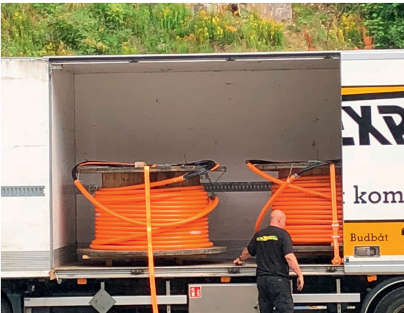
Umbilical subsea deck jumpers, 140m long with 15 hydraulic lines delivered in summer 2018, to a North sea project.
