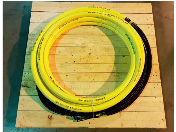
12 short umbilicals with 6 hydraulic lines installed on Gullfaks Topside Control unit. Planning to replace a total of 170 umbilical on Gullfaks A, B and C.
